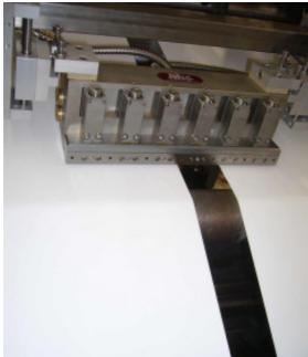
The coating heads are carried by solid precision brackets and can therefore place exactly relative to your product. This is crucial for optimum coating results and ensures simple setup with reproducible application.
