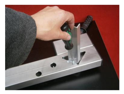
Fix it with two M4 screw. Adjust the guide before fixing the screws so that you can push the edge protector through the EVV-2 without hit the frame of the device.
