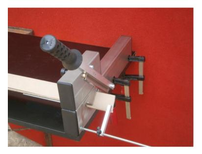
If you positioned the edge protector to the desired position, release the safety pin with pulling its knob.
