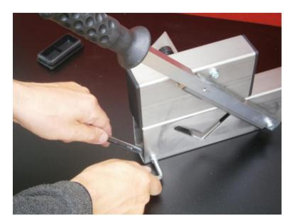
Remove the screw from the steel profile. (This screw is to secure the end position of the cutting knife. Do not remove this screw if you don't want to use the paper stop.)
