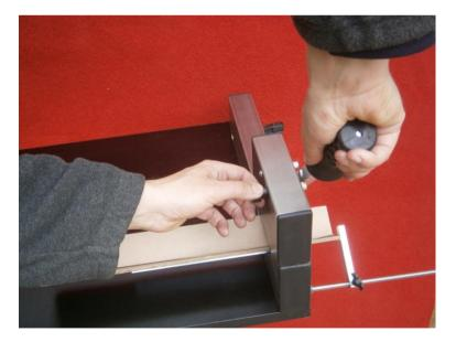
Then press down the handle of the machine to cut the profile. Move the handle upwards so long as it'll be fixed again in this upper position.
